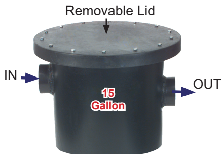
15 gallon tank (17.25" dia. x 15.5" H with 1.5" IPS inlet / outlet)
